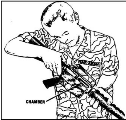
Figure 071-311-2025-3. Inspecting the chamber
