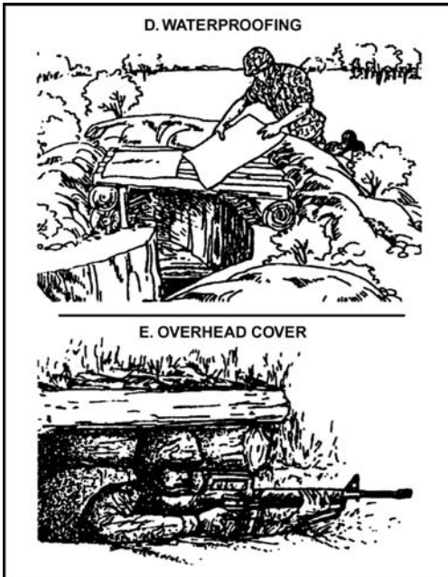
Figure 071-326-5703-5. Constructing overhead cover (continued)
