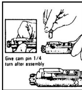
Figure 071-311-2025-28. Replacing the bolt cam pin
