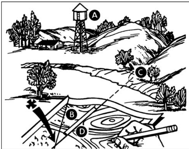
Figure 071-329-1015-3. Resection without a compass continued
